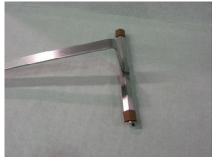
Apply silicon gasket 0.5" from sides
