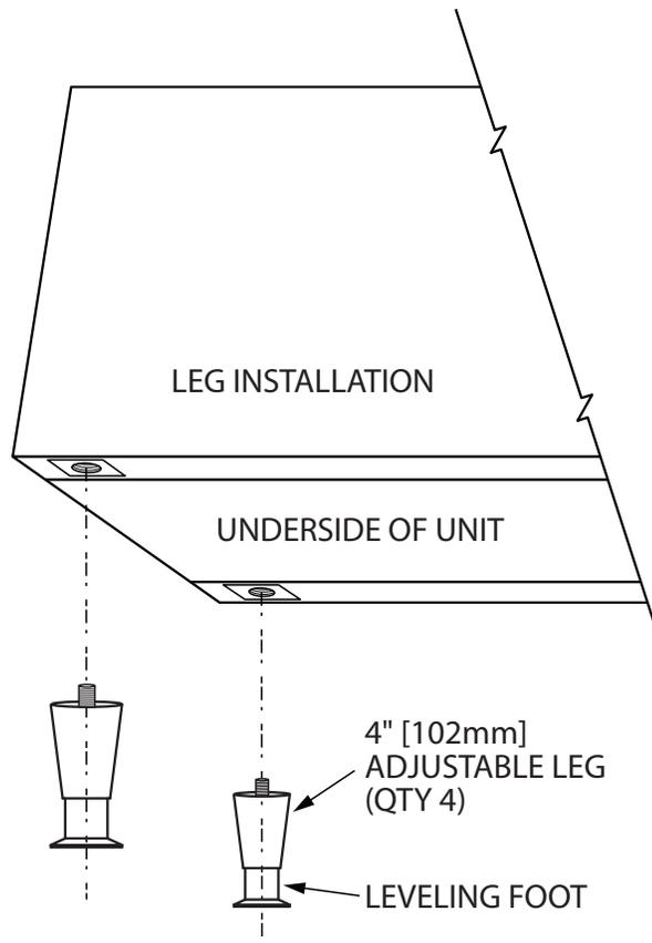
Level the appliance by adjustment of leveling bolts or legs. Use a spirit level and check for level four ways; across front and back, then down left and right edges. Level any adjacent units to the first. A griddle may not rest evenly on the appliance body if it is not properly leveled.
