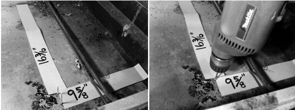
Left: Location of two holes marked by matchsticks for clarity Right: Drilling of holes
