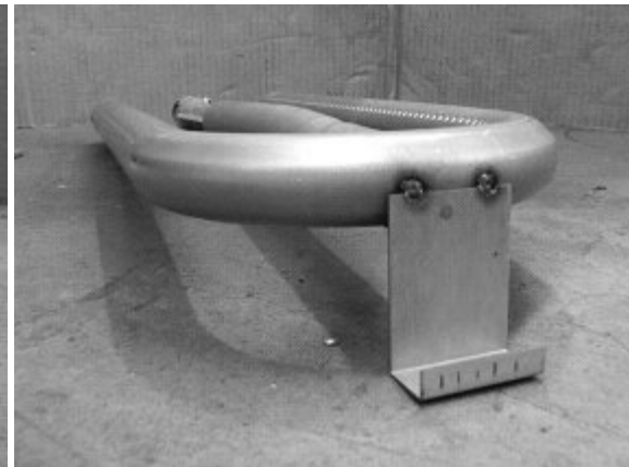
Left: Old burner with shorter bracket. Do not install this burner. Right: New burner with taller bracket, mounted to oven bottom. Install this burner.
