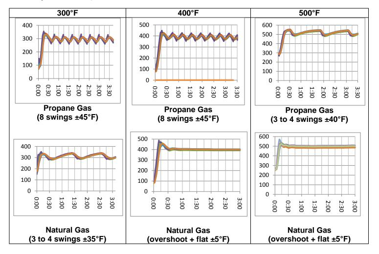
**NOTE**: The temperature stabilization at 400°F thermostat setting will happen after 45 minutes.
