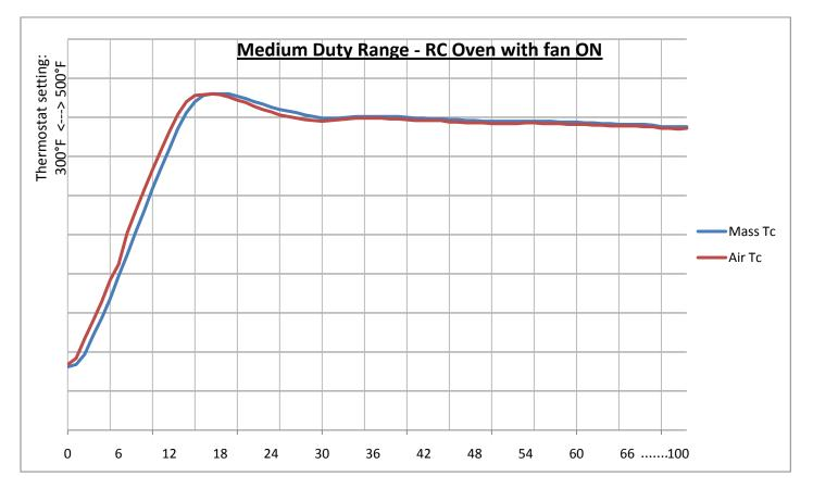
**Example** of typical curve pattern at different temperature settings in **Convection RC Ovens**:
