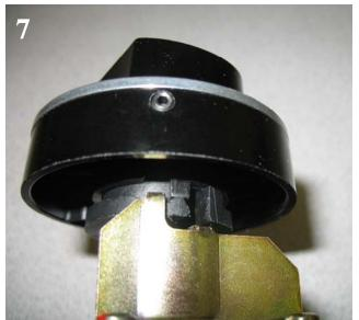
To shut down all gas to pilots and burners, loosen the knob set screw and gently pull knob off and proceed to figure 8.
