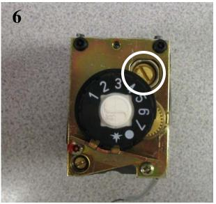
No adjustment should be made to the screw circled above.
