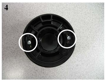
To calibrate the Thermostat, use the two screws on the knob. The factory preset position has the screws centered in the slots. The total range for adjustment is 30 degrees F. (± 15°F from midpoint setting)
