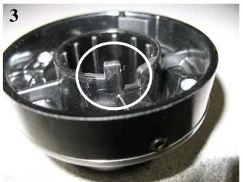
The tab must be intact on the knob For the knob to properly stop as shown in figure 2. If the tab is missing the knob will continue to turn until the pilots are extinguished. If the tab is damaged or missing, replace the knob. (See <u>NOTE#1</u>)
