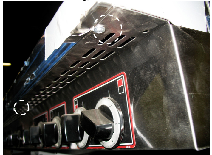
2. Next, remove the screws above the knobs.
