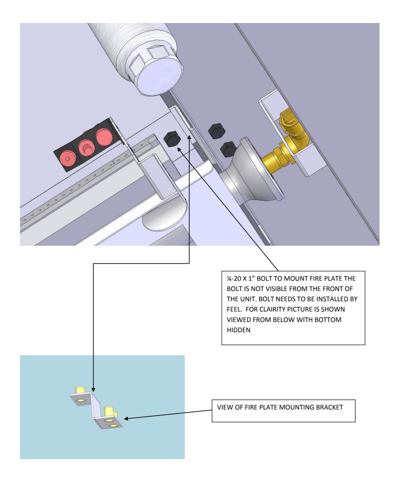
OVEN BURNER MAY NEED TO BE REMOVED TO ALLOW ROOM TO ATTACH FIRE PLATE. OVEN BURNER CAN BE REMOVED BY REMOVING ORIFICE BRACKET. THEN THE BURNER AND BURNER REST CAN BE PULLED OUT OF THE FRONT OF THE UNIT.
