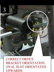
**Install the Pilot** to the bottom of the burner box.
