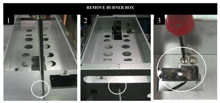
To remove the burner box, unscrew the orifice bracket from the box. The orifice bracket should be accessed with a 8" Robertson #2 screwdriver by gently lifting the front of the burner box once the front and rear mounting screws have been removed and the pilot is unscrewed.
