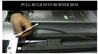
**2.11 Return Griddle Plate:** Position the griddle on the unit to allow for access to the bulb shield. Reinsert the thermostat bulbs into the shields and tighten down the shield nuts. Insure that the bulbs are inserted completely to the stop post located in the shield's channel.
