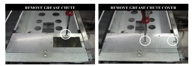
**1.9 Remove Grease Drawer Shield.** For Griddle plate sections exceeding 12" the grease drawer shield will be located on the right most burner box containing the grease chute. The shield is mounted via two screws. *Save the Grease Drawer Shield for installation on Field Kit burner boxes.*
