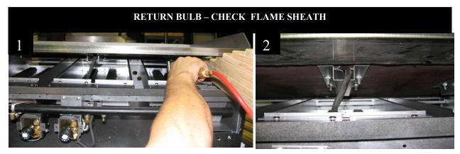
Position flame sheath to cover the thermostat wire length from the bulb shield. As the griddle is lowered into position insure that the excess bulb wire is drawn out of the burner box ands into the valve area in order to not get pinched by the griddle. To do this lower the griddle to 1" spacing and draw all excess bulb wire length into the valve area.
