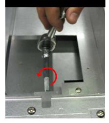
**2.8 Install Field Kit Baffles.** Mount one baffle to *each* side of the burner box via two screws as shown below. When installed correctly, the semi-circular notch on the high flange of the baffle should line up with the pilot to allow the pilot flame access to the main burner.
