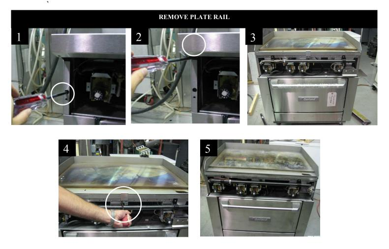
**1.4 Lift front portion of Griddle Plate.** Caution Thermostat Bulbs are mounted to the bottom of plate. Removal of Griddle Plate will cause permanent Thermostat damage if bulbs are not loosened and removed.
