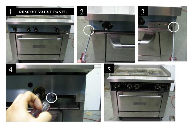
**1.3 Remove Plate Rail and Valve Panel End Caps**. Each End Cap is mounted via two screws located at the top and bottom of the rear flange. Uninstalling the Valve Panel End Caps first will allow the end caps and the Plate Rail to be removed in one step. Remove plate rail support located beneath the plate rail.
