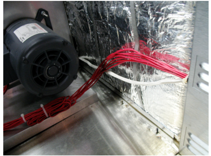
8. Then lift on the panel to remove it to reveal the white thermostat capillary sheathing.
