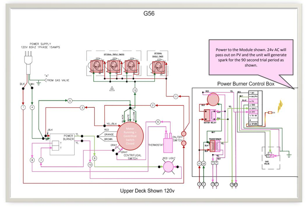
Unit Plugged in, Switch On, With a Call for Heat shown (Spark at module)
