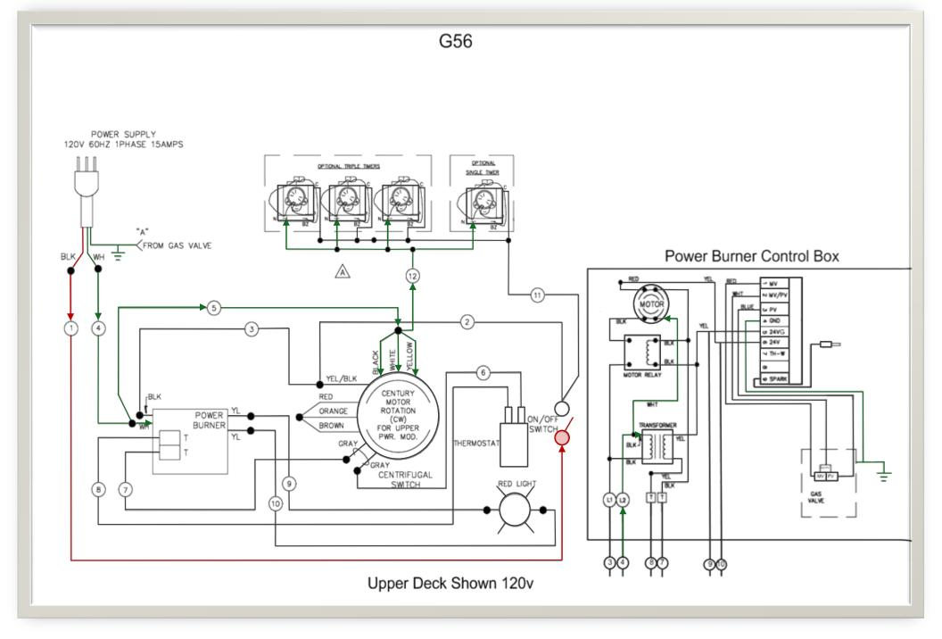
Unit Plugged in, Switch Off shown
