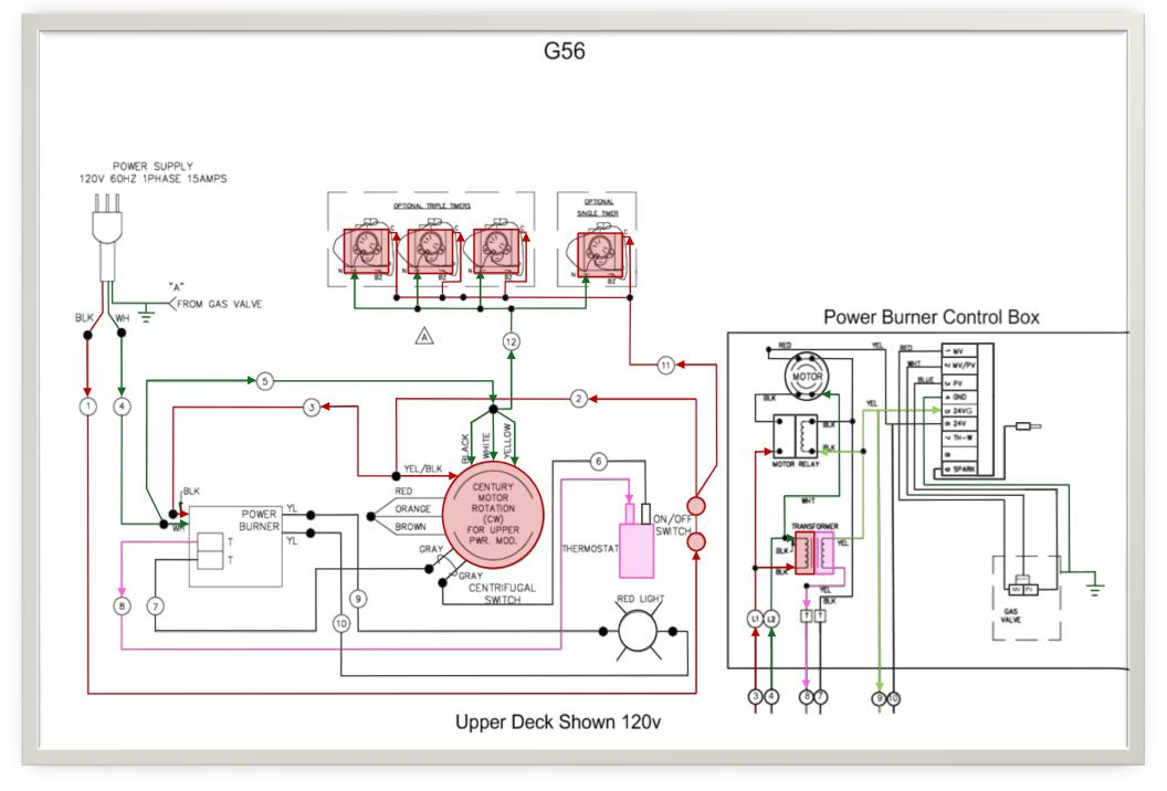
Unit Plugged in, Switch On, No Call for Heat shown
