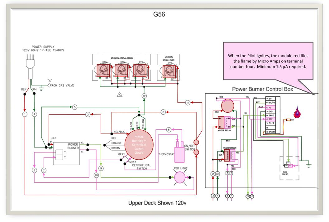
Unit Plugged in, Switch On, With a Call for Heat shown (Pilot lit)
