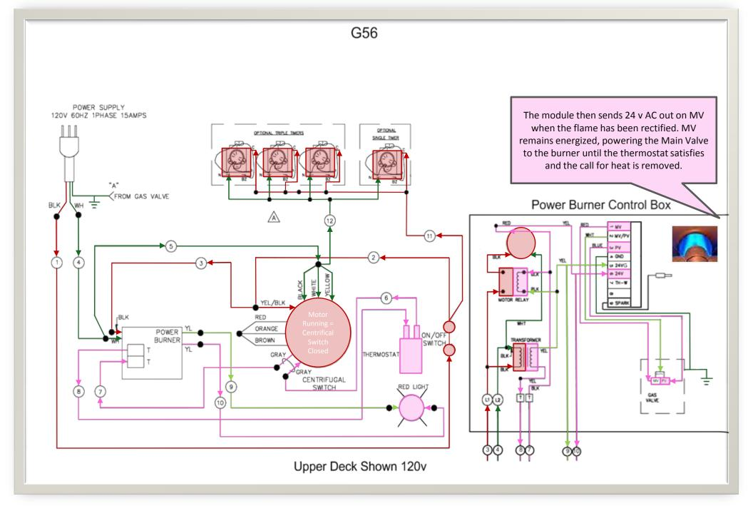
Unit Plugged in, Switch On, With a Call for Heat shown (Main burner lit)
