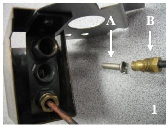
When assembling the Pilot, the pilot orifice (a) interlocks with the grooved ferrule (b).
