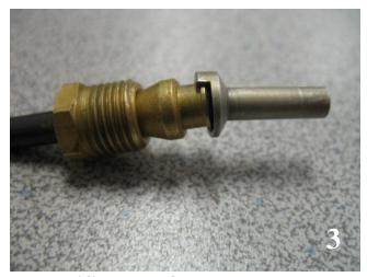
The orifice and ferrule can be interlocked prior to insertion, to verify they will seat properly within the pilot assembly.
