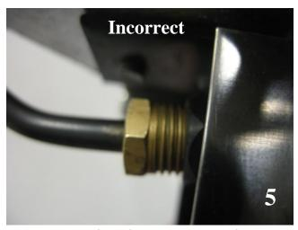
When the pilot is assembled incorrectly, approximately 4 threads will be shown.
