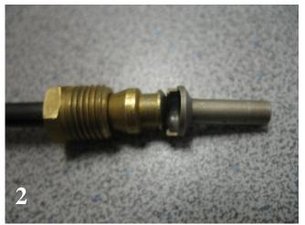
When installed incorrectly, the lip prevents the ferrule from seating completely with the orifice. This will have a negative effect on the pilot flame and needs to be corrected.
