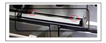
Below the burners in this section, a deflector crumb tray is installed on a slight angle to deflect any spilled liquids into the crumb tray to the left.
