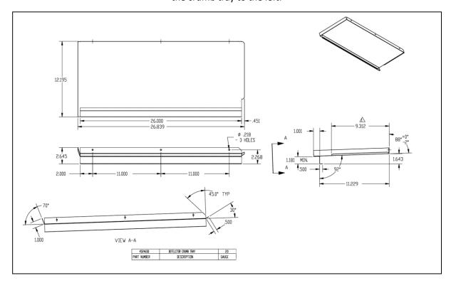
The Deflector Crumb Tray is located as shown below (item 5) and it should be cleaned as needed by removing the top grates and burners and wiping toward the crumb tray to the left, which can then be removed for cleaning.
