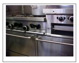
Note the tabs holding the false front in place
