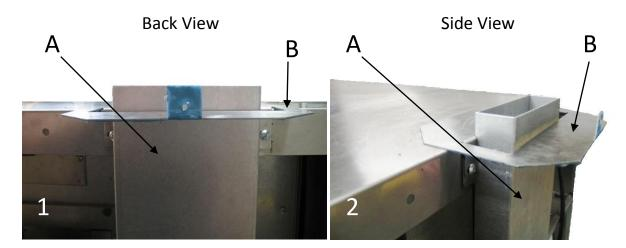
After removing the Flu (A – stacked flu shown, single flu installation follows the same procedure) by removing the 2 Philips screws and installing the Flu adapter (B – Remove protective coating before installation [shown for contrast]) the unit should appear as above.
