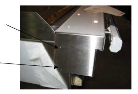
2. Clean front lip of griddle, on both sides, very well with alcohol or solvent.
