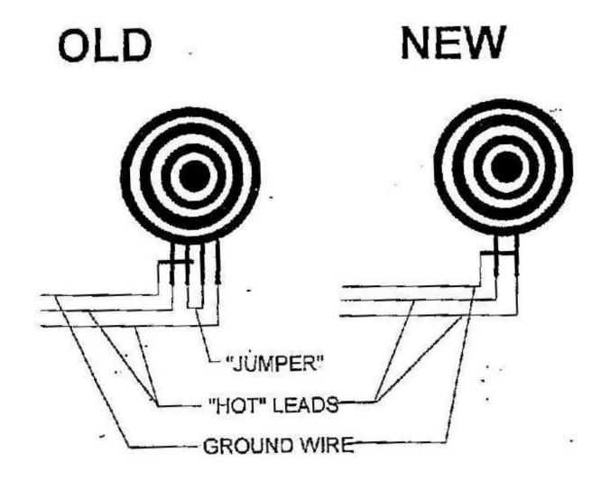
WHEN INSTALLING NEW ELEMENT, ELIMINATE "JUMPER"
