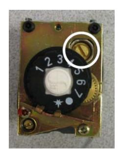
Garland uses a fixed drilled orifice to regulate the first stage in the SIT Control as shown below.
