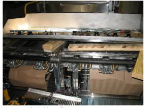
Use 2x4's and 4x4's to block up griddle, **be sure to use the sides of the range base for strength and stability**. \*use caution not to pinch the capillaries while lifting and lowering\*
