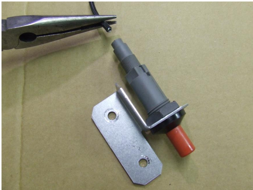
Detach igniter from original pilot assembly. The igniter will be reused with a new pilot assembly
