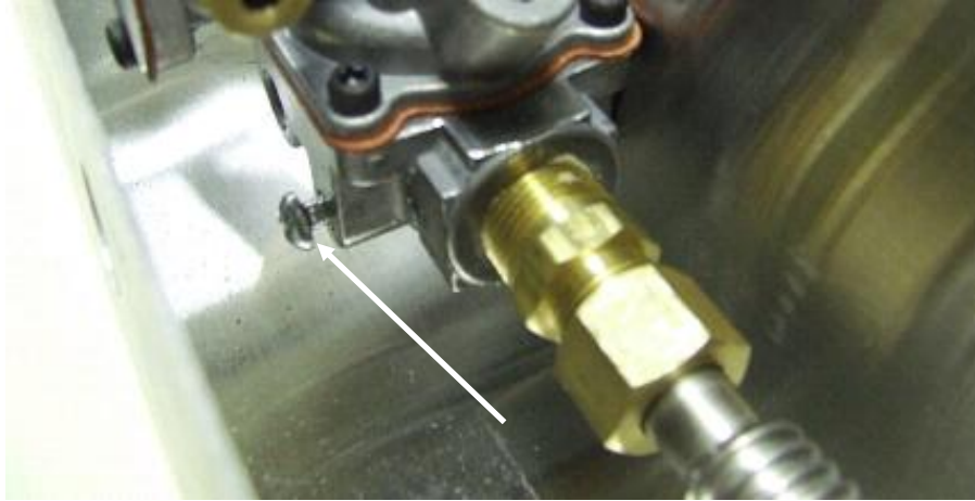
Attaching bolt inserted through hole in valve indicated by arrow
