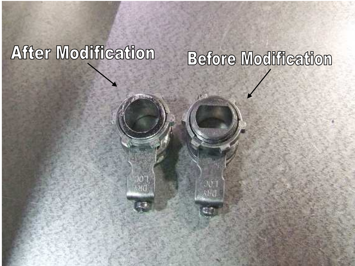
Before / After Comparison of modified BX Connector
