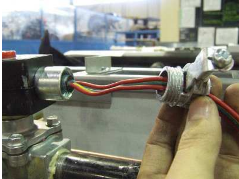
Modified BX Connector to Solenoid Valve
