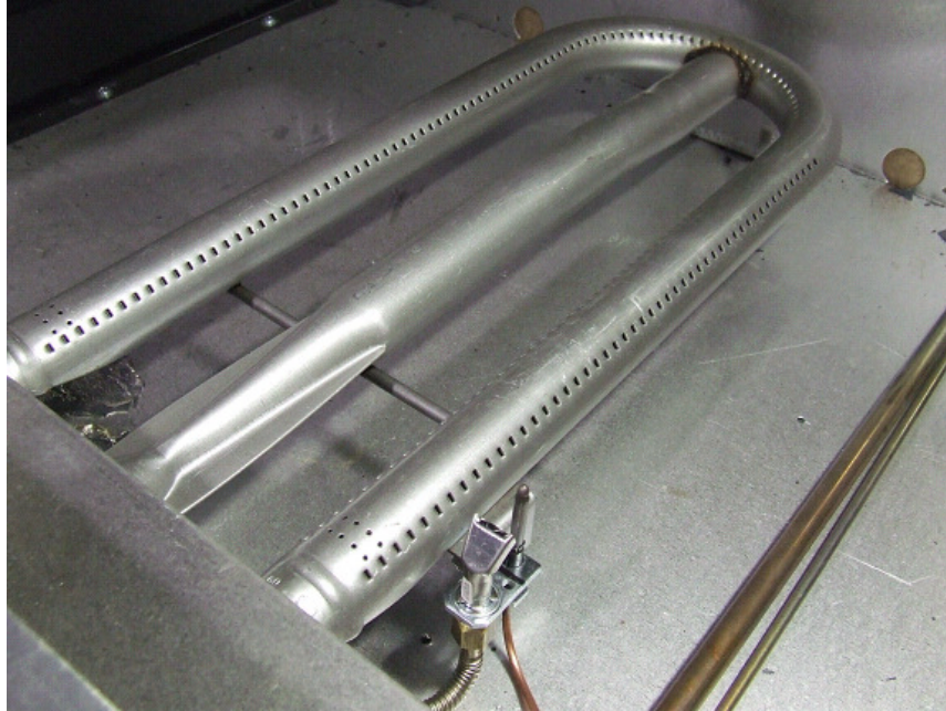
New welded bracket burner installed.
