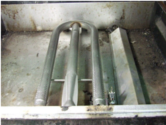
Left: Burner installed with no aeration plate Right: Burner uninstalled, no aeration plate models. Tall bracket at end
