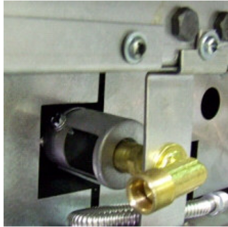
Orifice inserted straight into burner opening
