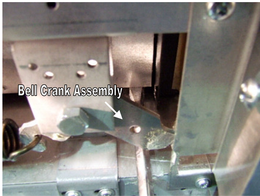
Insertion of screwdriver underneath bell crank assembly and air shield
