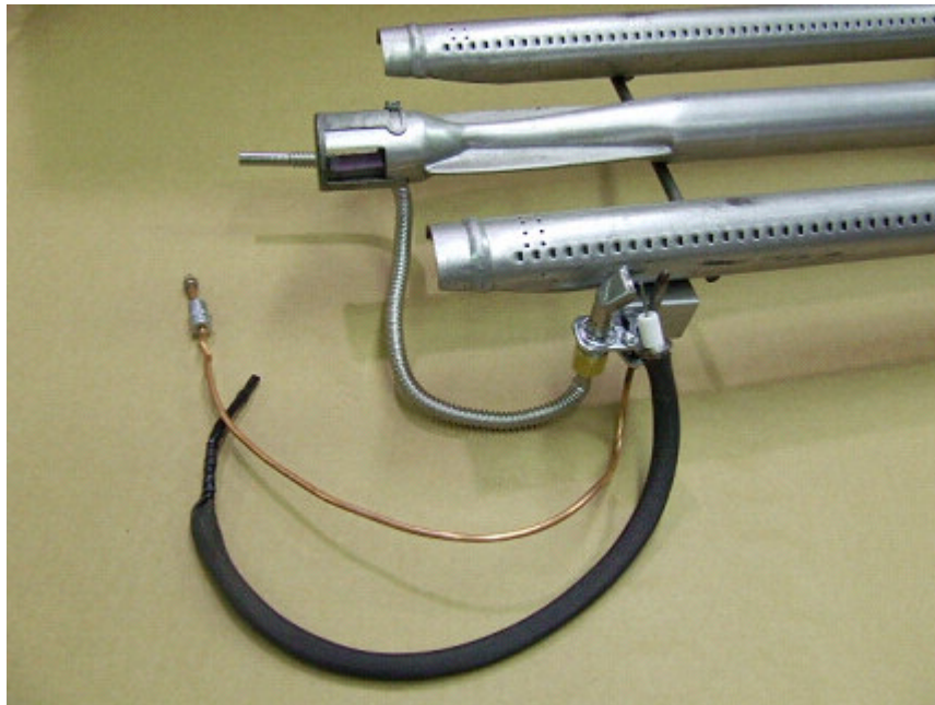
New pilot assembly attached to welded bracket on new burner.
