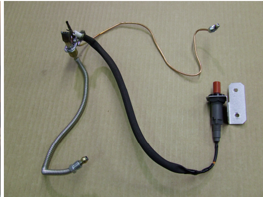
Left: Pilot assembly with bracket mounted to oven floor Right: Pilot assembly with bracket removed
