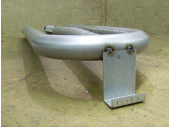
Left: Lower oven cavity after removal of front shields Right: Original burner with single welded bracket at end, will not be reinstalled
