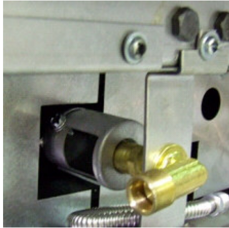
Orifice inserted straight into burner opening
