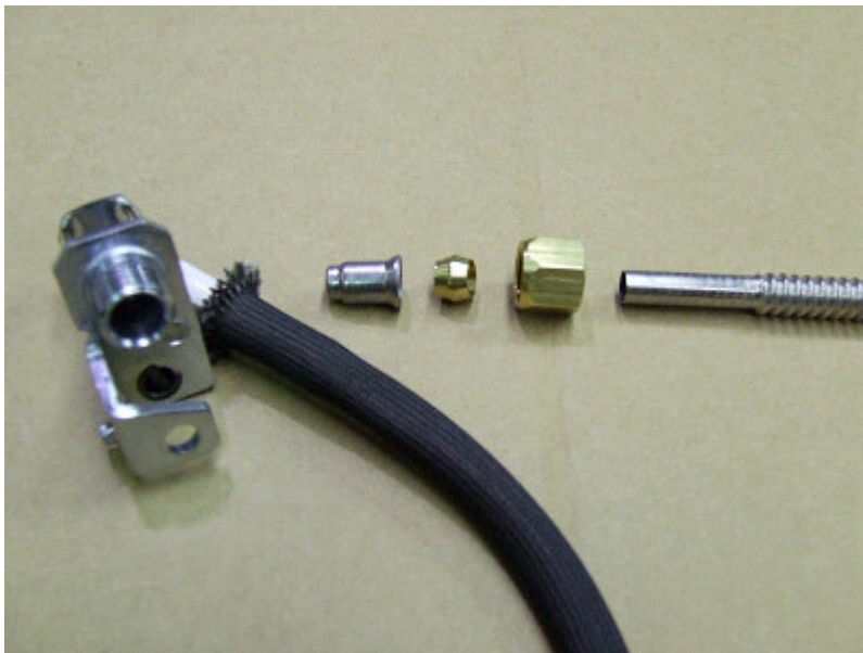
Nut on new pilot assembly unscrewed, revealing orifice and ferrule.
